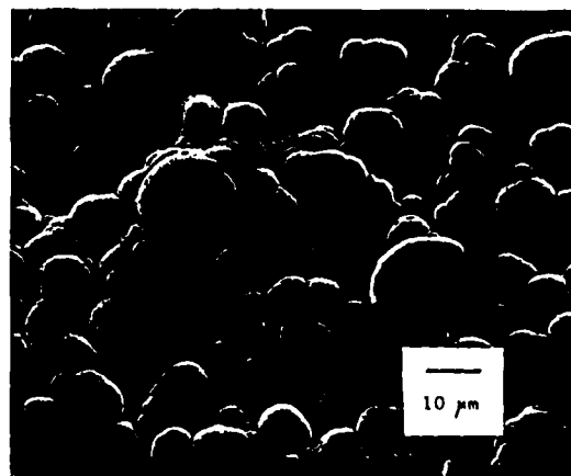
Figure 1. SEM micrograph of a PMT film on phosphated 430SS. The film was deposited on a 11mm dia RDE from 0.5M 3MT/0.1M TBATFB in propylene carbonate at a current of 60mA and a rotation rate of 100 RPM. The total charge passed was 15 mC/cm 2 .
