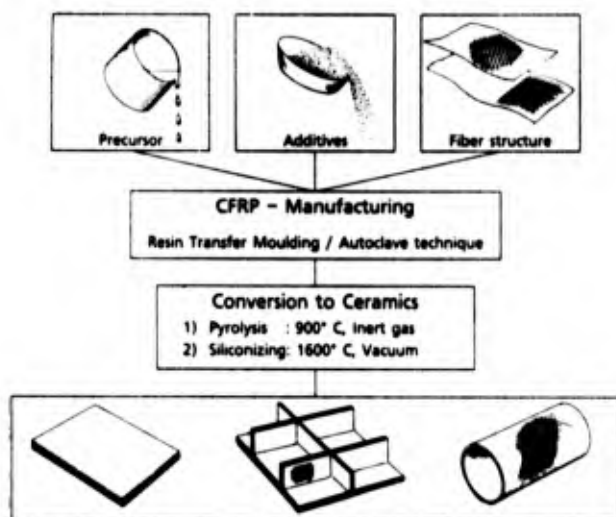
Figure 5: Schematic Illustration of the Liquid Infiltration Process
