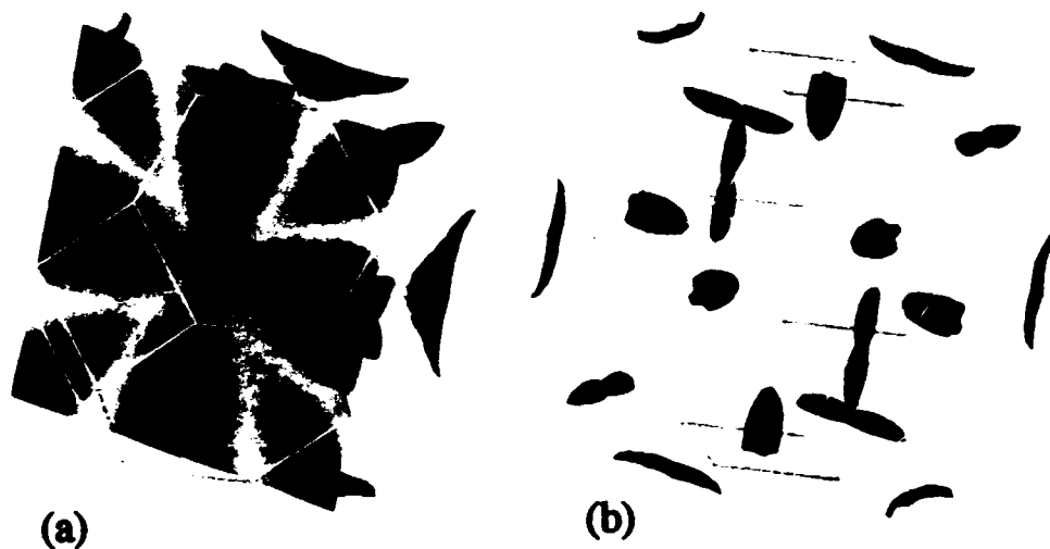
Figure 2. (a) Gray-scale contour plot of the first conduction band for silicon on the {100} plane; (b) Energy isosurfaces at E = 0.2 eV.
