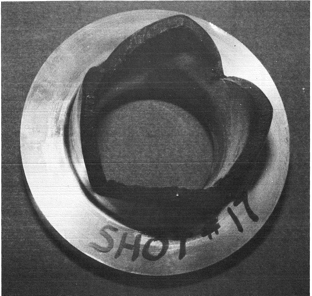
Figure 14. Posttest photo of 304SS shaped diaphragm, Test No. 17, 3,280 bars.
