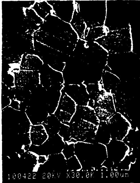
Figure 18 High magnification images of the polished and thermally etched surface of the 0.048 volume fraction, 18.6 aspect ratio composite.
