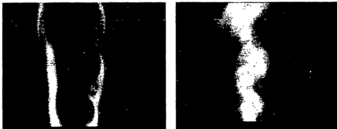
Fig. 1: Simultaneous single-shot two-dimensional fluorescence signal distribution of OH (left) and doped NO (right) in a turbulent H 2 /air diffusion flame
