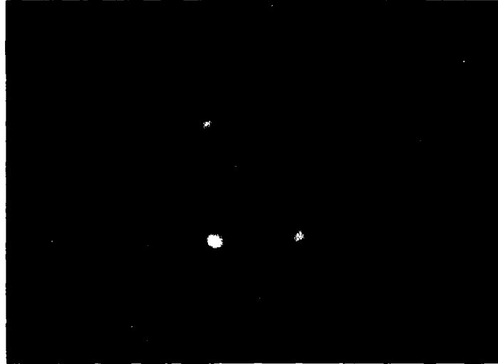
Figure 5 Electron diffraction pattern of the porous Si layer.
