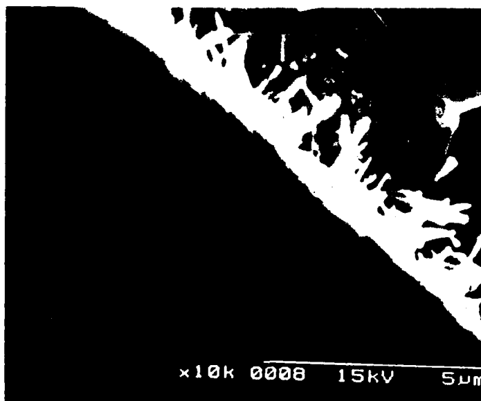
Figure 4 SM1240/Ti-6-4 Interface Carbon and TiB x layers, reaction zone and TiB needles
