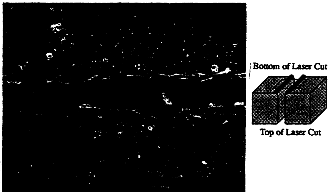
Figure 12.1. SEM micrograph of the cut exit of a 2 mm thick section of the 6061/ \text{Al}_2\text{O}_3 /20p composite cut at 15 cm/s.
