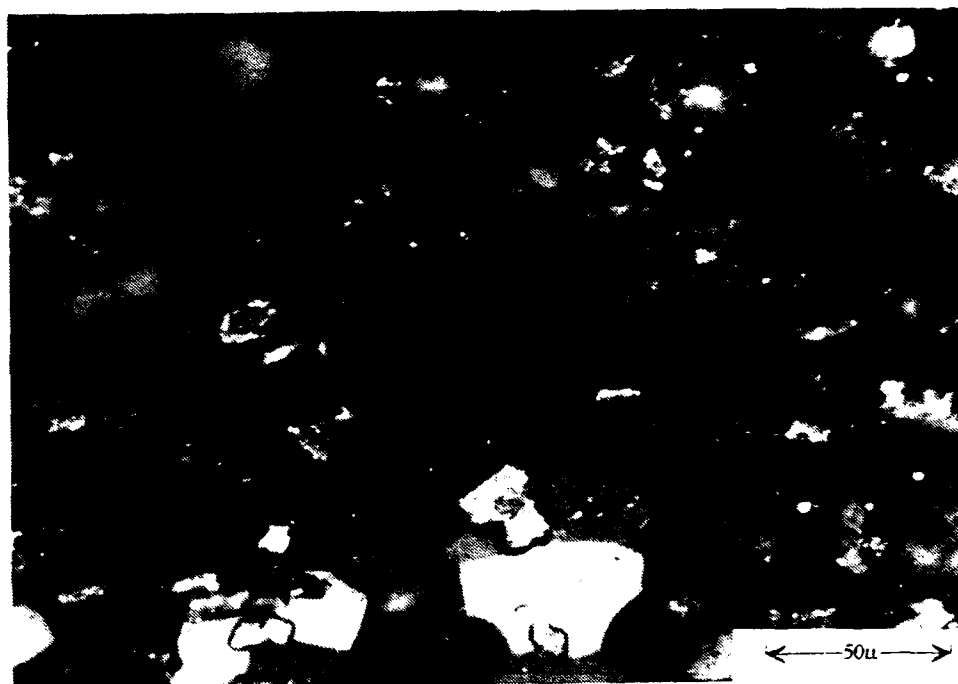
Figure 33. The microstructure of a rolled and solution heat treated 6061 - 20 vol. pct. \text{Al}_2\text{O}_3 composite illustrating complete recrystallization via PSN. Solution heat treatment was for one hour at 560^\circ\text{C} . Anodized and viewed under crossed polars.
