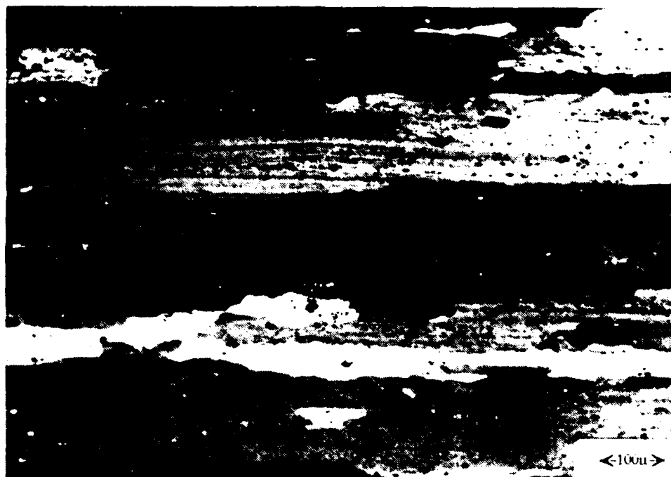
Figure 13. As-received 6061 Al-T6 plate, illustrating the elongated grain structure (grains \approx 1\text{mm} in length). The structure also shows inclusions aligned with the rolling direction.
