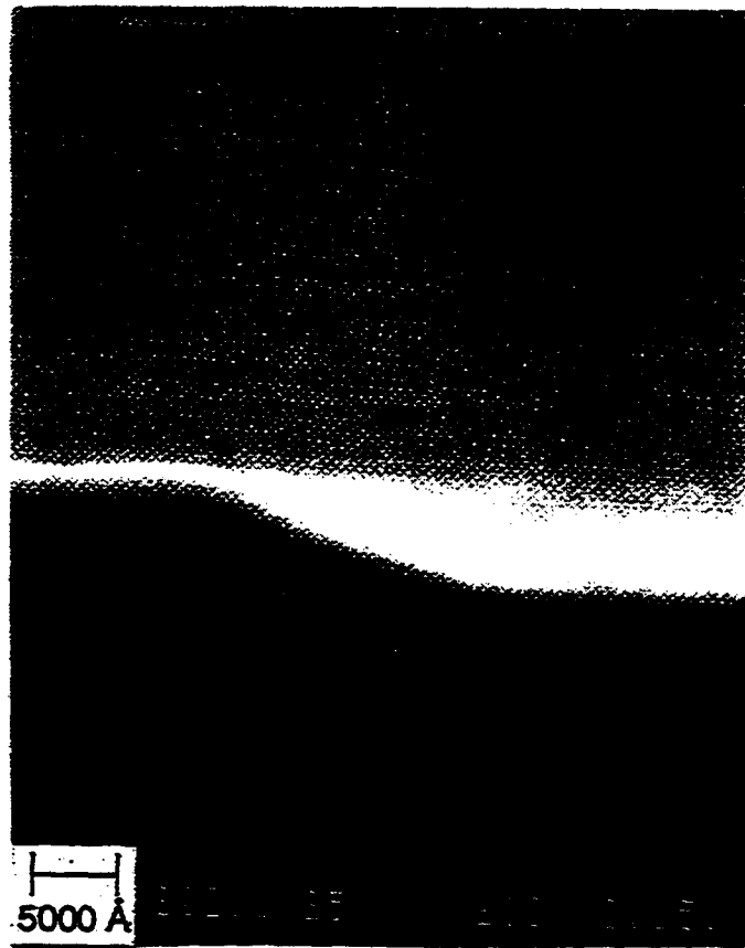
Figure 6.3 A close-up SEM photo of grating profile shows that the depth of the trenches is about 940 Å. The grating edges are not sharp.
