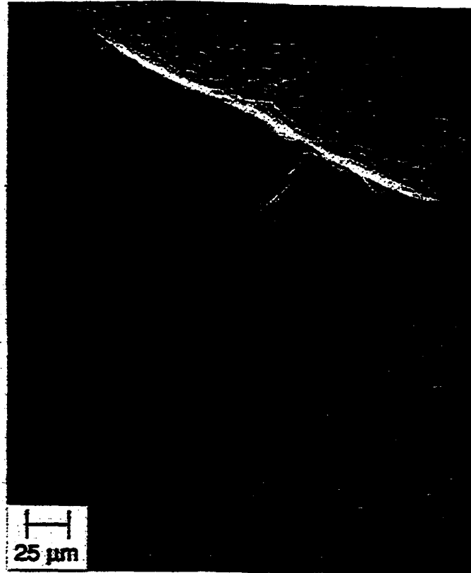
Figure 6.6 During imaging, the transmitted acoustic signal became unstable and the image quality was permanently degraded. Upon inspection in the SEM, the tip was found to be fractured apparently along crystallographic planes.
