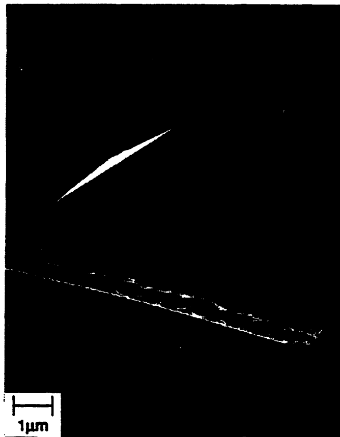
Figure 2.8 Unsharpened pyramidal tips can be formed integrally on AFM cantilevers. Their unsharpened radii of curvature is approximately 500 Å.
