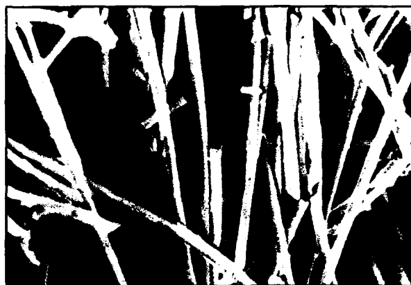
Fig. 2 — SEM image of copper-coated microtubules at a magnification of 6,000 \times
