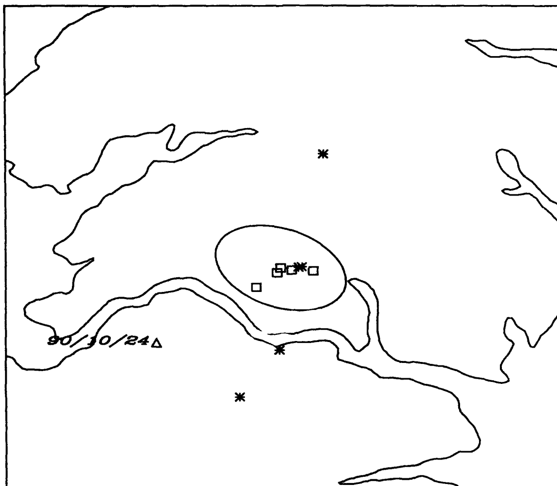
Figure 7: The asterisk symbols show the two station locations based on the readings of the analysts of the event 92/12/31. The 90% confidence ellipse and the 3 station solutions from Figure 6 are included for comparison. The location of the reference event 90/10/24 is indicated with a triangle. The distance horizontally and vertically across the map is 100 km.
