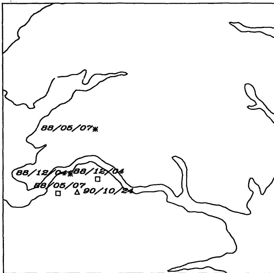
Figure 8: The asterisk symbols show the two station locations based on the readings of an analyst of the events on 88/05/07 and 88/12/04. The locations of the JEDs for these two events are marked with squared symbols. The location of the reference event 90/10/24 is indicated with a triangle. The distance horizontally and vertically across the map is 100 km.
