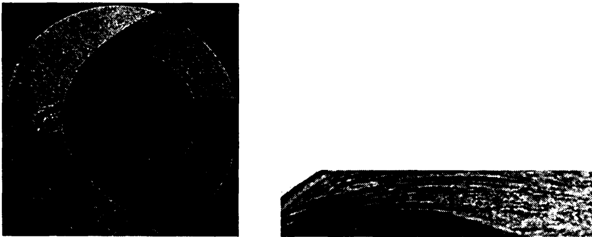
Fig. I.13. Resonantly-enhanced shadowgraph of CO 2 flow over a sphere of 4 in diameter. Free-stream condition: CO 2 , 3.55 km/s, 0.081 kg/m 3 , 11.27 MJ/kg.
