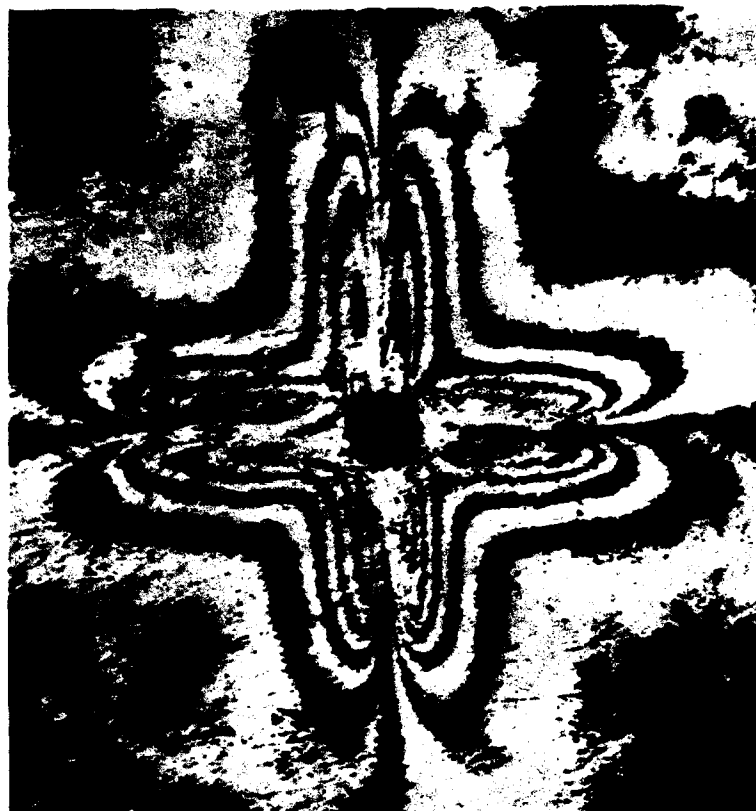
Fig. 15. Inner strains formed by pressing on the 001-face of KRS-5.
