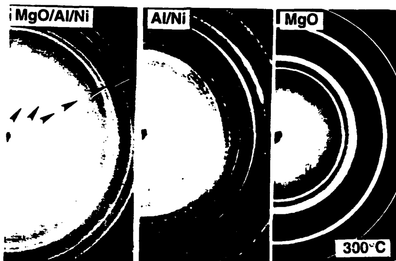
Figure 5. SAD patterns of films after annealing at 300°C for 100s.
