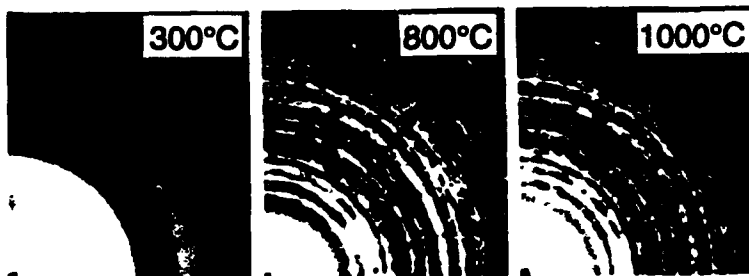
Figure 12. Electron diffraction patterns of a baseline 500A-thick ZrO 2 film, annealed simultaneously with the NiAl/ZrO 2 film. The structure is monoclinic at both 800 and 1000°C.
