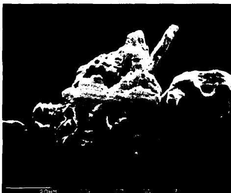
Figure 5 SEM photograph showing Ni-particles (magn. plug orange 110.25 hours operating time)
