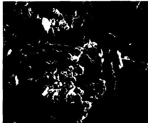
Figure 4 SEM photograph of wear particles with different form and size (magn. plug orange 110h)
