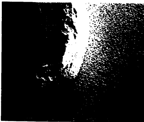
Figure 5 The SEM-photograph shows the cor- rosive attacked and poorly manu- factured contact surface 5 (S)
