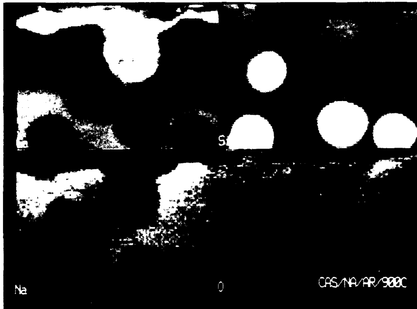
Figure 33. Advanced X-Ray Imaging of Reaction Zone in Coated SiC/CAS Heat Treated in Argon at 900° C (Shown in Figure 32)
