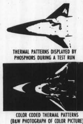
Figure 31. Thermal mapping (thermographic phosphors).
