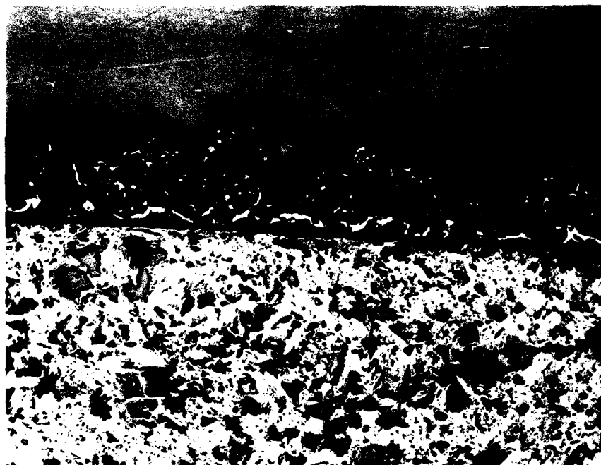
Figure 5. High-Density Coating of \text{TiB}_2 on Graphite, 100X
