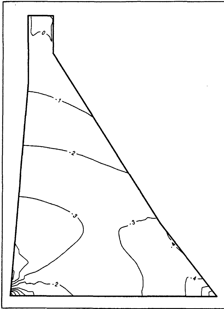
Figure 48. E_r/E_c = 1.75 , horizontal stress contours
