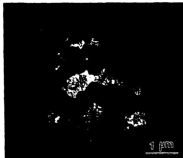
FIG. 9. Dark-field TEM micrograph of GaN film grown on (111) Si, using a cubic reflection, highlighting the zinc-blende phase in the material.
