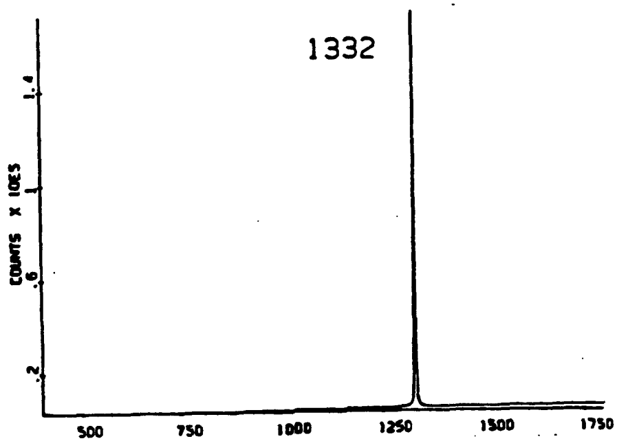
Figure 5. Raman spectrum of a diamond crystal 9 .
