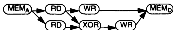
Figure 7 Antecedence Graph of a RAID Level 5 Small-Write Operation. Given a block of data, this antecedence graph illustrates the ordering dependencies required to complete a RAID level 5 small-write operation as described in Figure 3(a). Actions include: allocation of memory; reading of old data and old parity; writing of new data; exclusive-or of old data, old parity, and new data to generate the new parity; the writing of new parity; and the deallocation of memory. Since context is not required, disk read operations (RD) do not indicate the logical object type, data or parity, being read. Because of this, error handlers for each of these actions can be constructed and executed independent of operation type.
