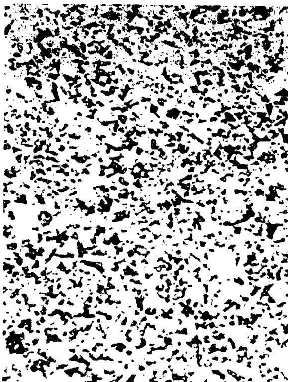
Figure 23. Representative photomicrograph of tungsten carbide material, as-polished at 1500X.
