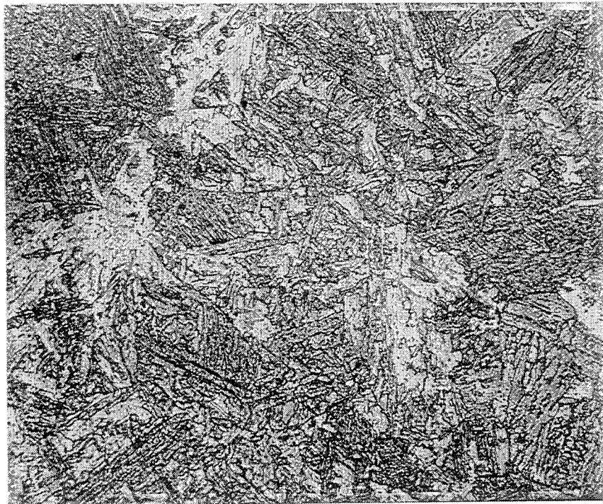
Figure 3.5 CS2AM Recrystallized Zone Bainite (500 X)
