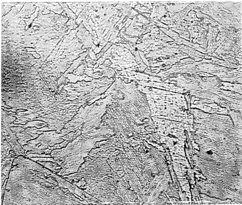
Figure 3.6 CS2AT Final Pass Bainite (500 X)
