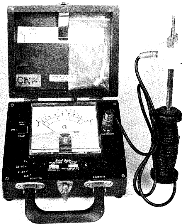
Delmhorst Moisture Detector. This detector determines moisture content of wood and related items used in the shipment and storage of ammunition. It has a detection range of up to 80 percent
