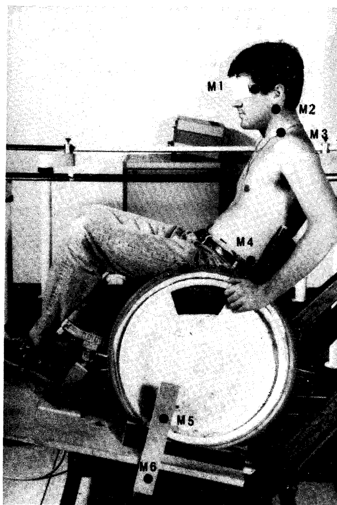
Figure 2. Subject equipped with markers in experimental situation. (M1: temporal bone; M2: maxillar-superior head rotation center; M3: inferior head rotation center; M4: iliac crest; M5: oscillating platform; M6: platform rotation axis).
