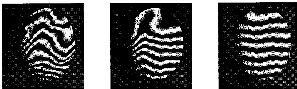
Figure 31. y -direction interferogram patterns for 5.4 cm - 3.6 cm, 3.6 cm - 1.8 cm, and 1.8 cm - 0.0 cm from the shear flow chamber (top view). The fringe separation is proportional to the wavefront slope in the y direction. Gas flow is from right to left. Helium velocity is 8.3 m/sec. Nitrogen velocity is 1.5 m/sec.
