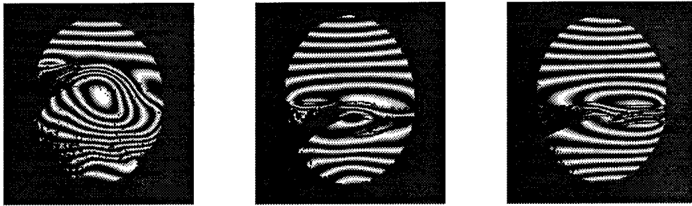
Figure 43. y -direction interferogram patterns for 5.4 cm - 3.6 cm, 3.6 cm - 1.8 cm, and 1.8 cm - 0.0 cm from the shear flow chamber (side view). The fringe separation is proportional to the wavefront slope in the y direction. Gas flow is from right to left. Helium velocity is 8.3 m/sec. Nitrogen velocity is 1.5 m/sec.
