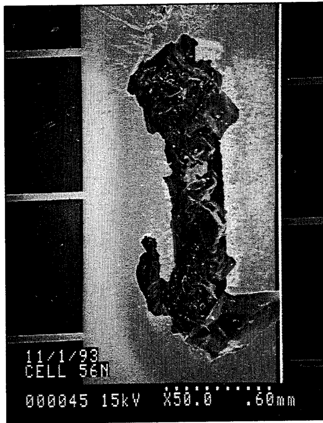
Figure 17. Typical fracture surface of modified N-side weld with Si divot.
