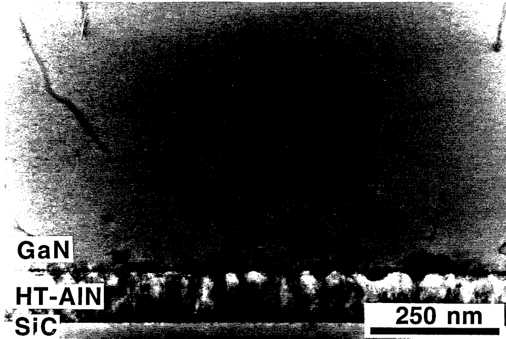
Figure 1. TEM micrograph of GaN grown on vicinal SiC(0001) Si at 950°C by OMVPE employing a high-temperature (1100°C) monocrystalline AlN buffer layer.
