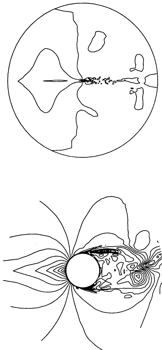
Figure 72: Re = 3,900 ; Instantaneous density ( \rho ) 144 \times 136 \times 48 Dynamic model simulation top : whole grid; bottom : cylinder vicinity
