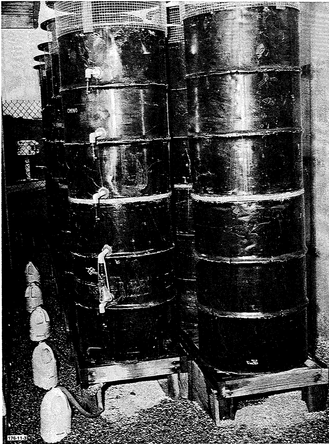
Figure 12. AOMC Lysimeter Setup.
