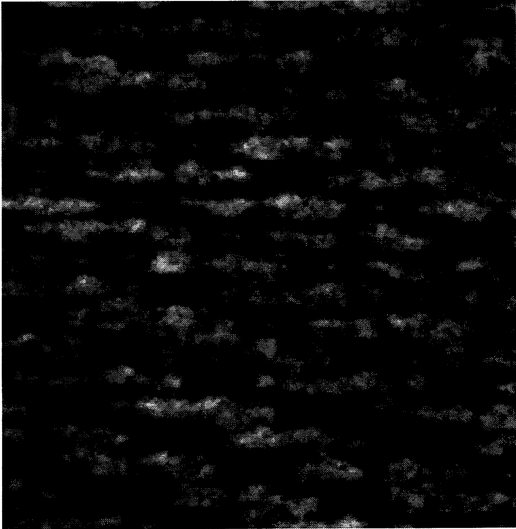
Figure 15. Amplitude plot from acoustic microscope scan of carbon-carbon composite plate. Pulse-echo mode using 25 MHz spherically focused piezoelectric transducer. Scan area 0.75"x 0.75".
