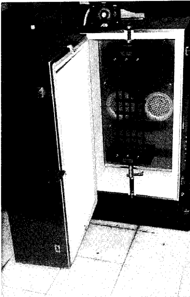
The Louisiana Transportation Research Center uses temperature-controlled creep testing equipment in a project for development of accelerated creep testing procedures for geosynthetics.
