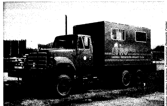
The Louisiana Electric Cone Penetrometer System (LECOPS) shown above has been implemented successfully in the field in connection with projects dealing with site investigation and pile capacity design and prediction. The LECOPS interior, shown below, is equipped with penetrometer probes, a depth encoder, and data acquisition hardware and software.
