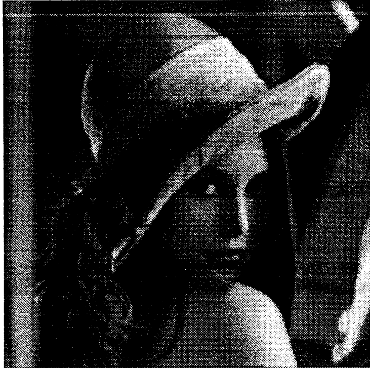
Figure 31b. Image with Lorentzian PSF of radius 1.0 pixels, condition number 138, and 5.0% Gaussian noise.
