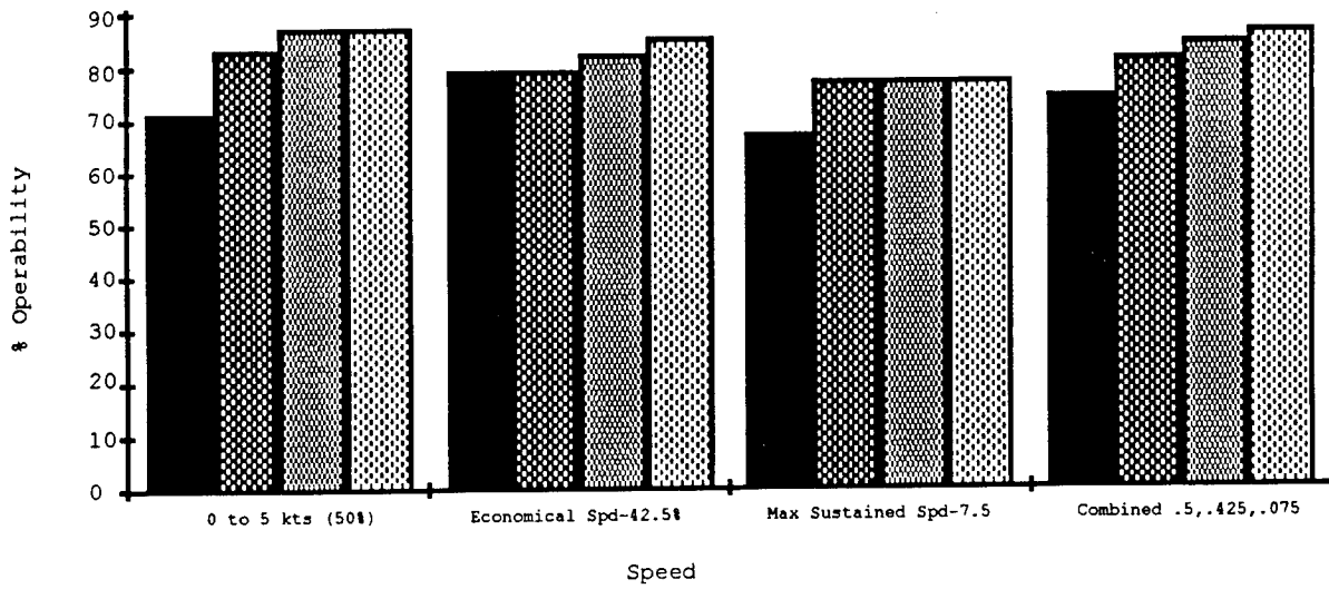
Figure 17 Speed Effect at Grid Point P-625 for USCGC 47-Ft, 82-Ft, 110-Ft Unstab & 110-Ft Stab; Base Criteria Set, Annual Wave Data; (File CG11F.grf)
