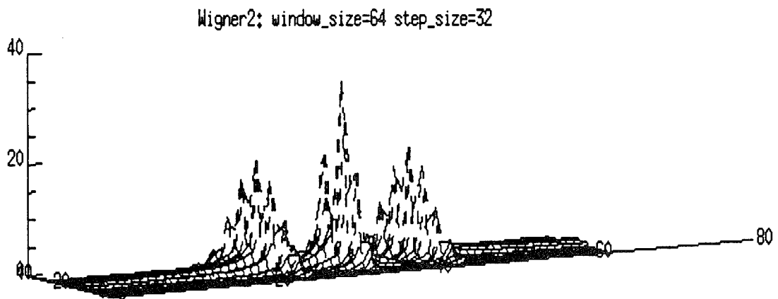
Figure 5. Sum of chirp(0.2,5,50) and chirp(0.2,5,-50), its STFT, and its WVD
