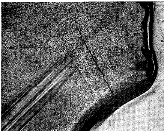
Figure 5. c) A cellulose-acetate replica of the disk surface, showing a crack
