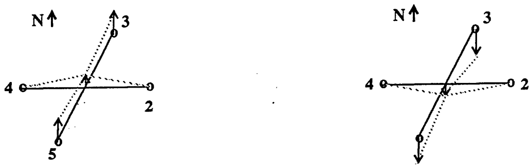
Figure 20.A.6 Inward/Outward transponder error raises/lowers depth of array 1-6m
