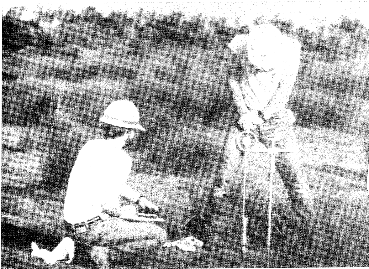
Figure 1. Field soil testing for vehicle mobility determination using the cone penetrometer
