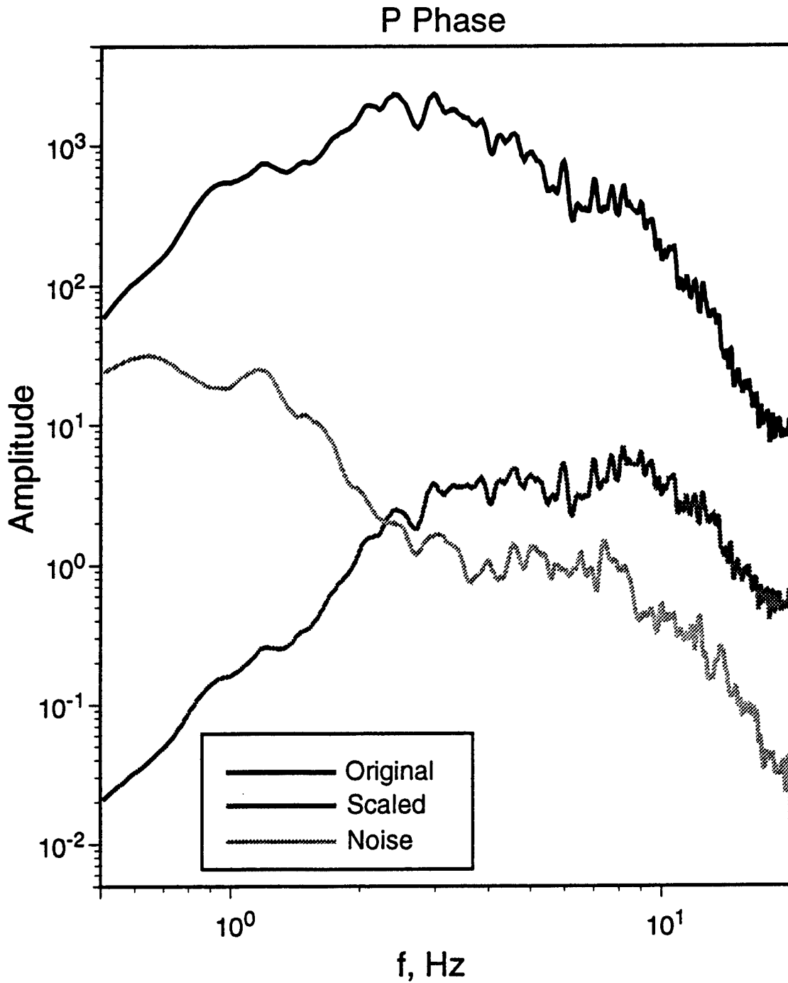
Figure 6. Comparison of regional P-wave Fourier spectra determined from ARA0 record of 10/24/90 NZ explosion before and after scaling to 1kt decoupled relative to spectrum of background noise.
