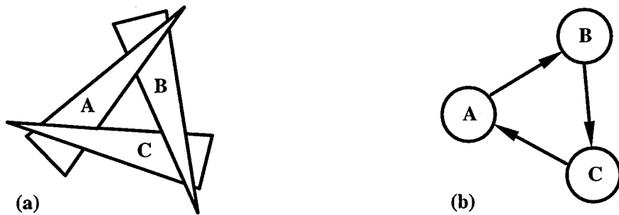
Figure 11: (a) A configuration of three objects and (b) its associated cyclic occlusion graph.
