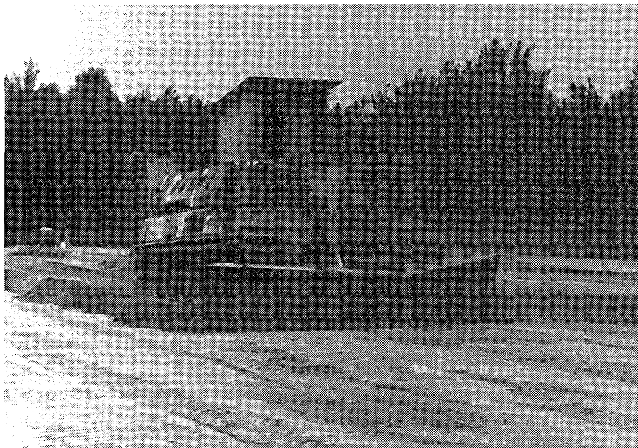
Figure 7. “V Plow” with Teeth Removed
