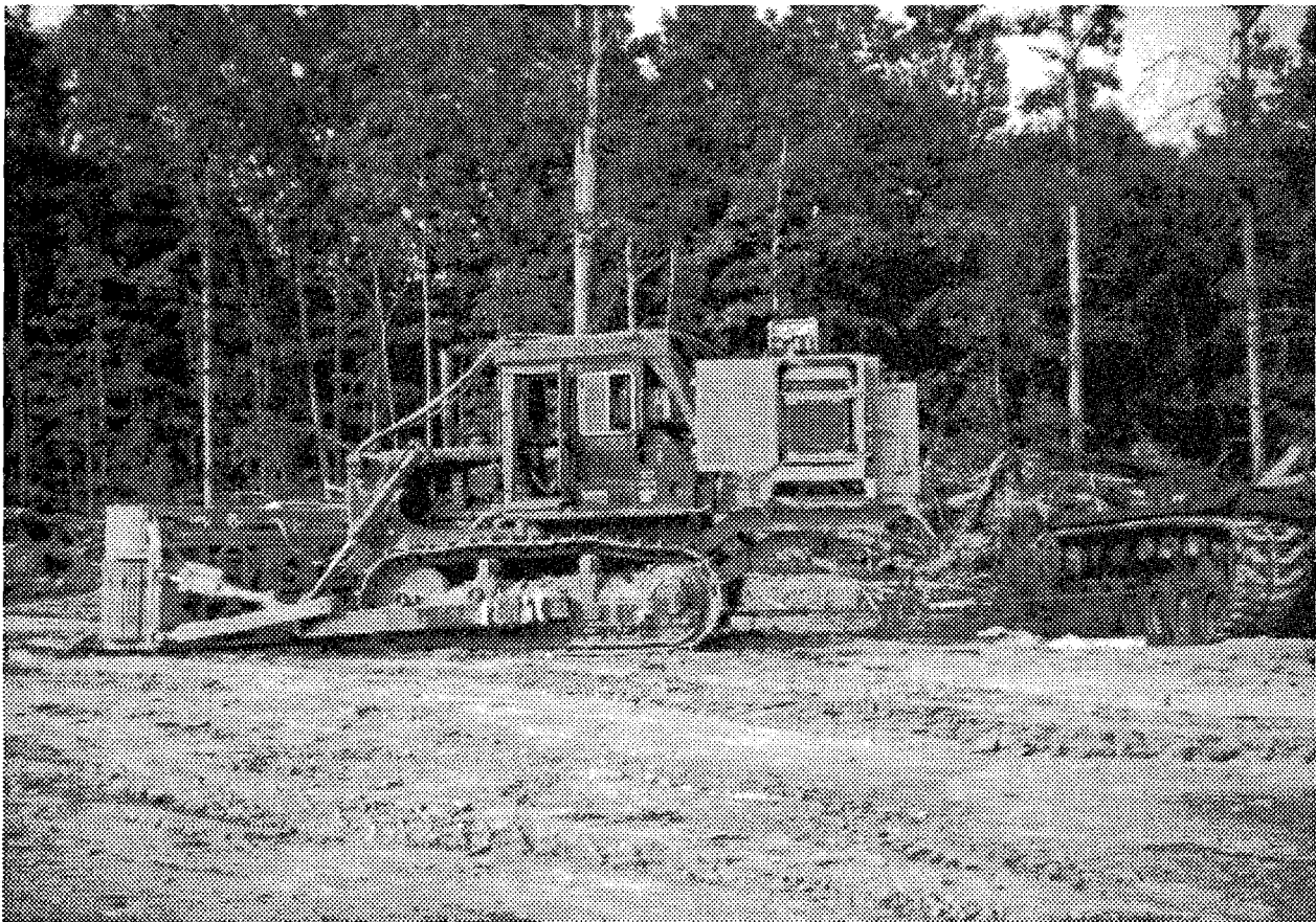
Figure 8. Pull Test with D7-G and Clausen Blade
