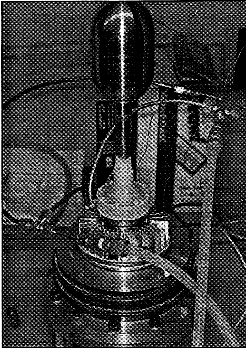
Figure 8. Frosted Cold Heat Exchanger
