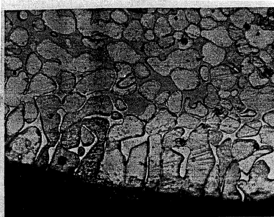
Figure 7a. Edge CIP rod 1/4"/hr at 1200°C- travel across page. 200X.
