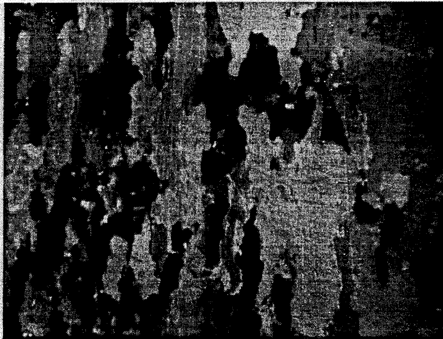
Figure 9. Ingot #4, sintered and float zoned 93% W CIP rod-travel down page. 100X
