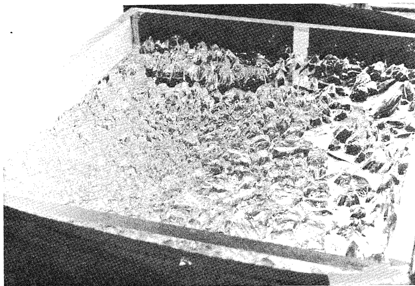
Figure 4. Ice crystals in the freshwater tank break away from each other as their grain boundaries melt (candle ice).
