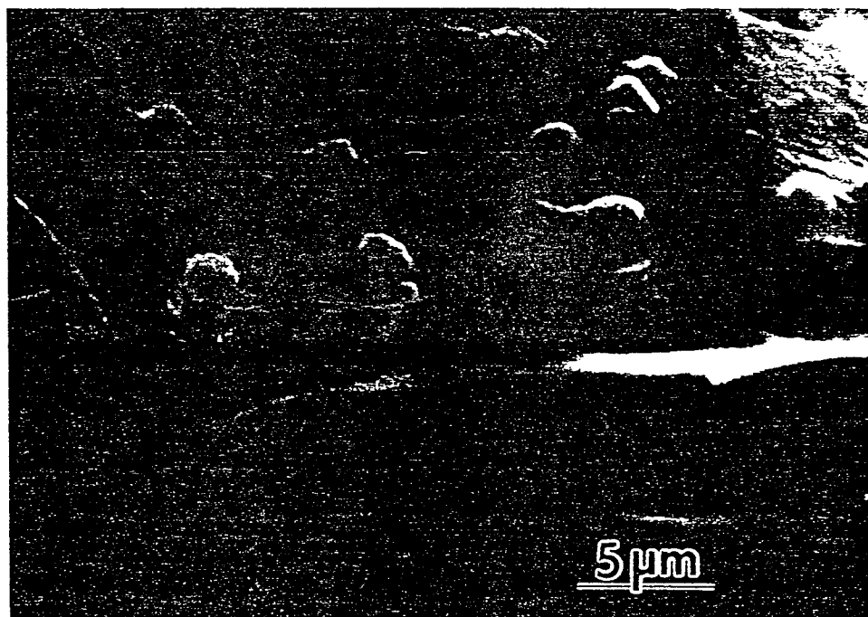
Fig. 4 - Scanning electron micrograph from the growing edge of the abalone nacre showing the nuclei and their distribution.
