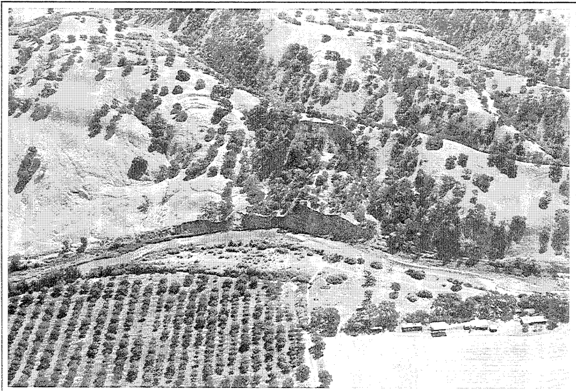
Figure 2.3 Sheet, Rill, Gully, and Channel Erosion Combined with Mass Wasting in the Source Zone of Cache Creek, CA
