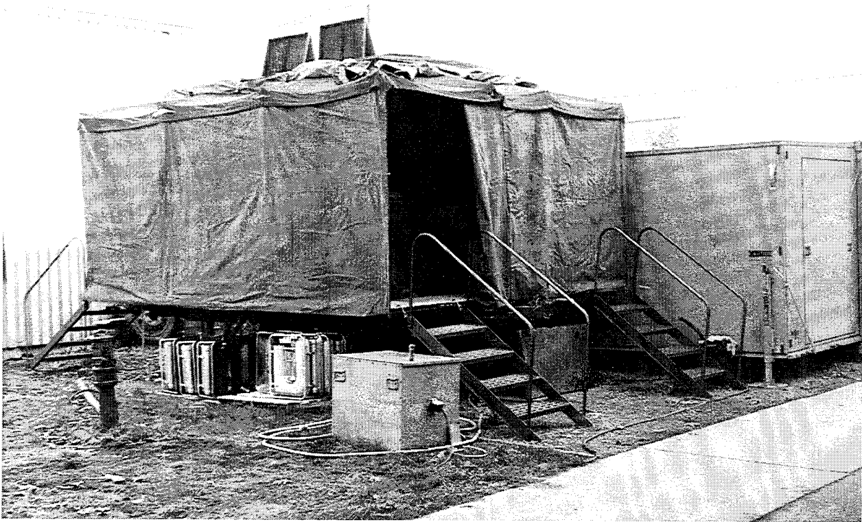
Figure 8. Permanent roof vent covers on the MKT, tied together for the installation of new roof vent covers.
