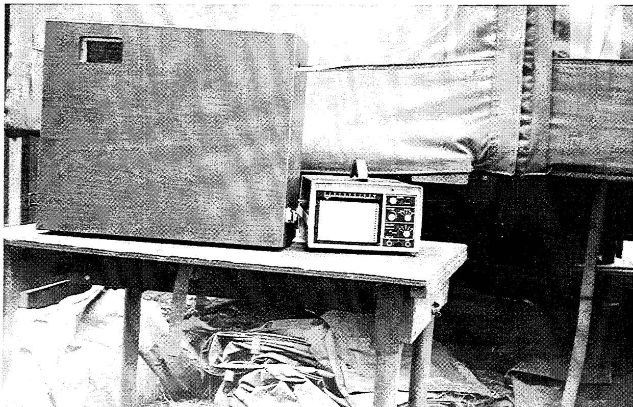
Figure 23. TGM 555 monitor and LINEAR chart recorder used for testing formaldehyde.
